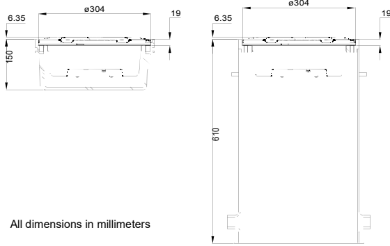
LRCL - Typical installation
