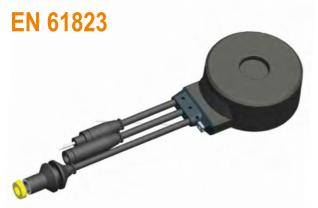
An Airfield Ground Lighting (AGL) transformer, also named isolation transformer, is typically installed in series circuits in airport approach line, runway, taxiway and other airport lighting systems to provide right amount of current to the low voltage lights respectively along the circuit and to ensure main circuit continuity in case of light failure.
